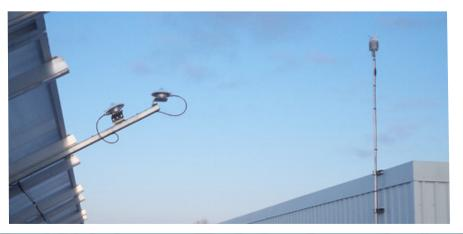
This weather station installation shows two radiation sensors, one at plane of array and one at GHI, as well as the Orion weather sensor module on the mast at right. This utility-scale Ontario, Canada solar energy project required our highest accuracy pyranometers.
