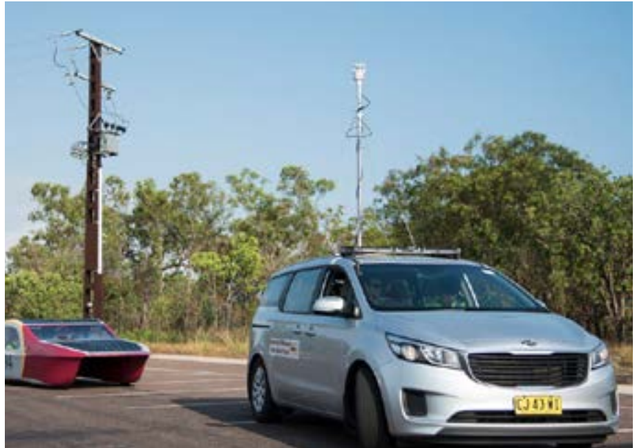
The all-in-one sensor head mounted on the support vehicle provided vital information throughout the 1,800-mile journey.
