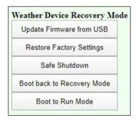
To upgrade the MicroServer firmware click on Update Firmware, then click Enter Recovery Mode to boot the MicroServer into the upgrade environment. Once in Recovery Mode click Update Firmware, click Choose File and select the firmware file.
