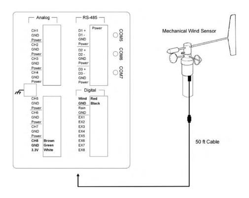
Using a #1 Straight Slot screwdriver, attach the wires from the end of the sensor cable to the green terminal block screws on the MicroServer as follows:
