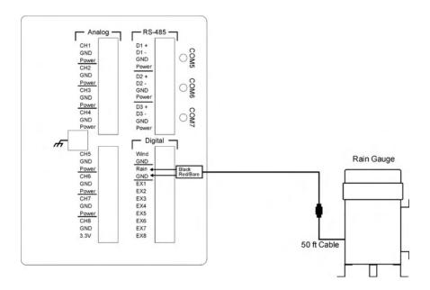
Using a #1 Straight Slot screwdriver, attach the wires from the end of the sensor cable to the green terminal block screws on the MicroServer as follows:
