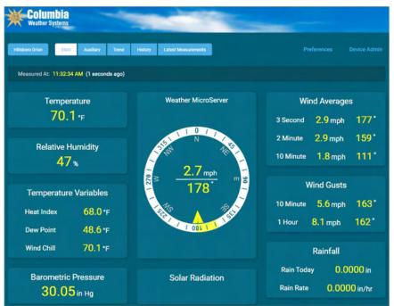
The Main Dashboard page displays the station name and the main parameters in the selected units.
