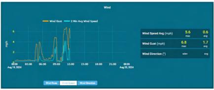
Wind Speed Trend – Displays Trend for 10-minute wind gust and 2minute average wind speed for the last 48 hours.
