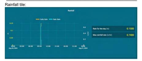
Displays trend data for Rain for the day and Rain Rate for the last 48 hours.
