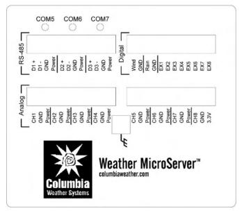
The Top Panel includes three RS485 Serial ports for sensor input and Modbus RTU interface, eight (8) Analog Channels available for additional sensors, a rain input channel for the tipping bucket rain gauge, and a wind speed input channel for a mechanical wind sensor.
