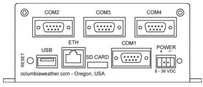
The MicroServer has four RS232 Serial ports, an Ethernet port, USB port, SD Card slot, reset button, and power connector.
