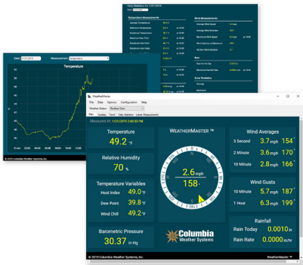
WeatherMaster™ Software provides real-time computer weather monitoring with display and automatic logging of parameters.
