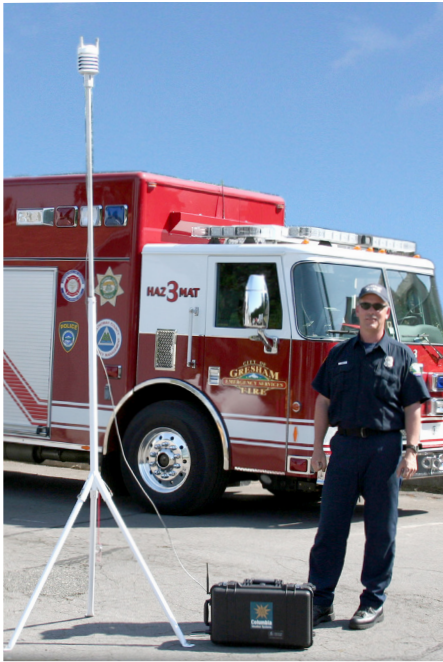
Portable Weather Stations, popular with HazMat teams and environmental researchers alike, offer a rapid-deployment option for short-term on-site weather monitoring.
