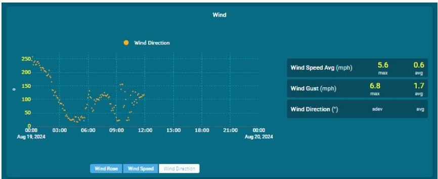
Wind Direction Trend – Displays a scatterplot of the wind direction 2-minute average.
