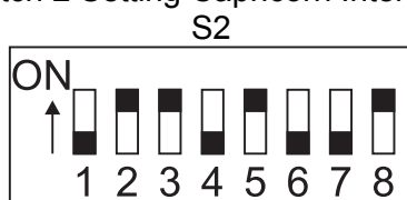
Figure 5: Switch 2 Setting Capricorn Interface as a DTE
