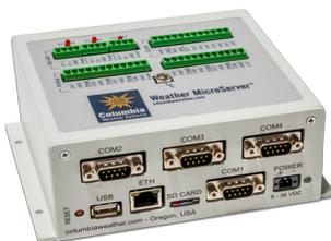
Four serial ports offer interface to the weather station and additional sensors such as visibility and ultrasonic wind sensors. Analog and digital channels available for additional sensor such as temperature, solar radiation, and rain gauge. The MicroServer provides real-time weather data to WeatherMaster software and the Display Console over the network. This allows users to simultaneously monitor the weather over the network.
