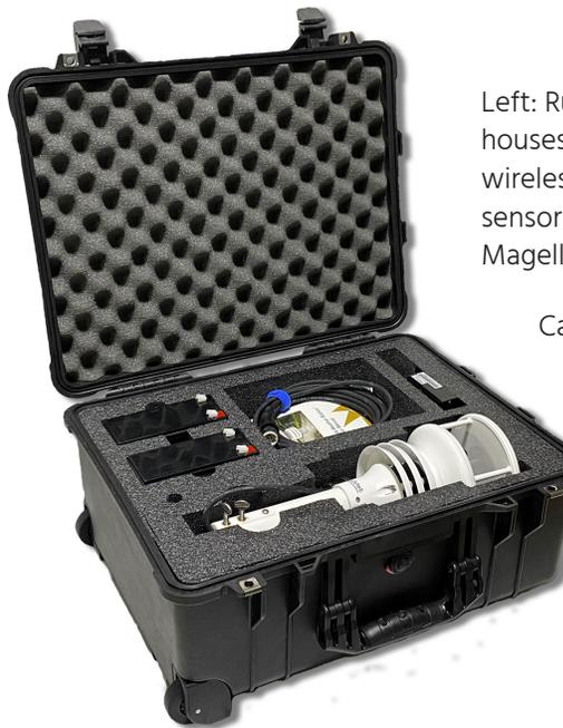
Left: Rugged, wheeled carrying case houses met sensors, batteries, and wireless transceiver with quick-connect sensor plug-in jacks. (Shown with Magellan MX500 sensor with GPS.)
