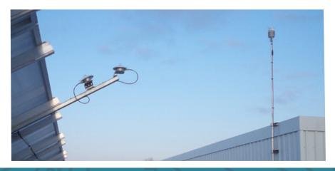
This weather station installation shows two radiation sensors, one at plane of array and one at GHI, as well as the Orion weather sensor module on the mast at right. This utility-scale Ontario, Canada solar energy project required our highest accuracy pyranometers.
