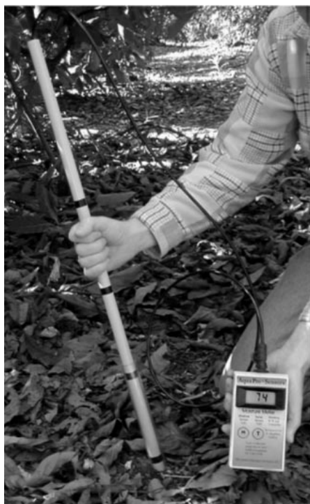
Portable Probe and Moisture Meter. Black bands are depth markings.
