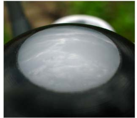
The self-cleaning convex lens is designed to accurately measure low-angle radiation coming directly from the sun in the morning and evening.
