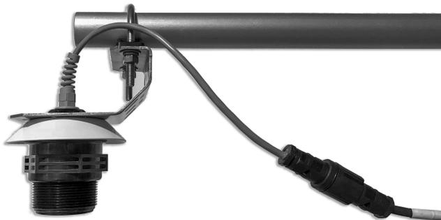
The Ultrasonic Snow Depth/Water Level Sensor transmits an ultrasonic pulsed sound wave through the air to meet a reflective object, such as snow. When the sound wave contacts the target, it bounces back toward the sensor. The sensor records the time required for the sound wave to travel to the target and return. Using the speed of sound, the sensor calculates the distance to the object.
