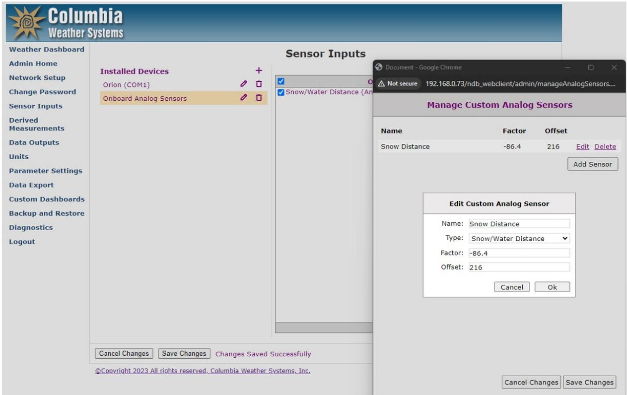
The Offset will vary from sensor to sensor due to calibration.
