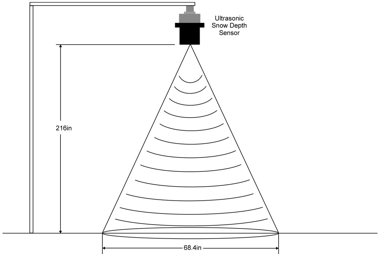
To avoid inaccurate readings the sensor should be mounted away from any obstructions in the measurement area.
