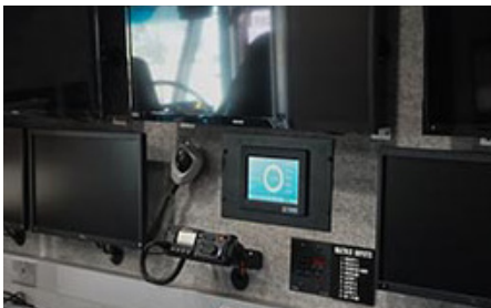
A panel mount Weather Display on the interior of the Mobile Command Center
