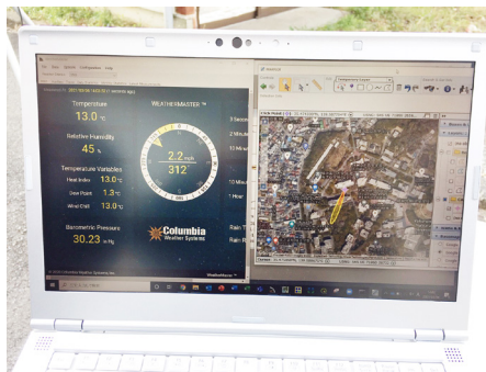
Plume modeling utilizing weather station data with ALOHA, transferred to Google Earth through Marplot. (Photos courtesy of Toyoaki Nakarai)
