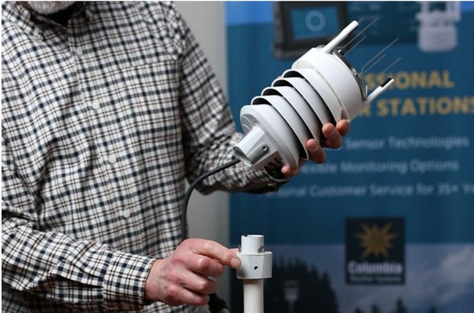
**2.** Loosen the three screws at the bottom of the sensor with the provided allen wrench (or screwdriver with allen adaptor) and slide out completely.
