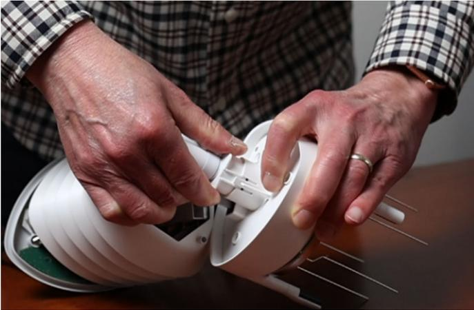
6. Connect the new PTU module by pushing in firmly. Replace the top, re-connect the flat ribbon cable, replace the base and tighten the three bottom screws.
