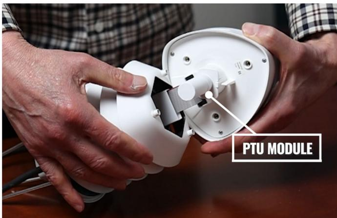
5. Release the small white flap and remove the PTU module.
